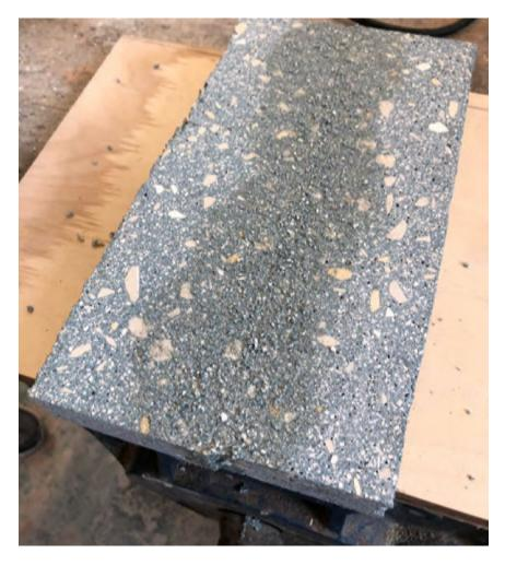
4. Allow the material to fully cure, the repair dust will increase the curing time, lower ambient temperatures will also effect the cure time.
