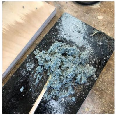
1. When mixed use a pallet knife or spatula to apply the material over the join.
